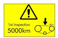
This sticker is supposed to be located on the sun visor of the van. It will have to be removed after completion of the first inspection.
