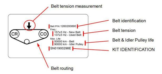
The sticker (above) showing the belt tension value and life time has been **doubled** in all drive kits effective April 2015. One sticker can be located on the vehicle (engine compartment or left door area and the second one may be placed in the maintenance book of the Refrigeration Unit or of the vehicle.
